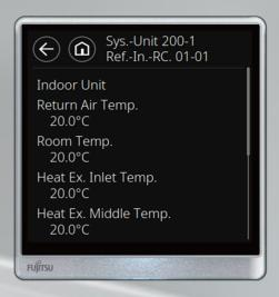
When connected to H Series split models (see bulletin 185 for details) and VRF systems, service information can be viewed on the controller for both the indoor and outdoor unit. This information includes:
