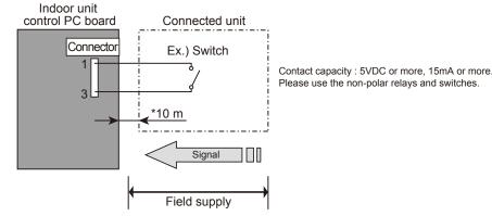
\* Make the distance from the PC board to the connected unit within 10m.
