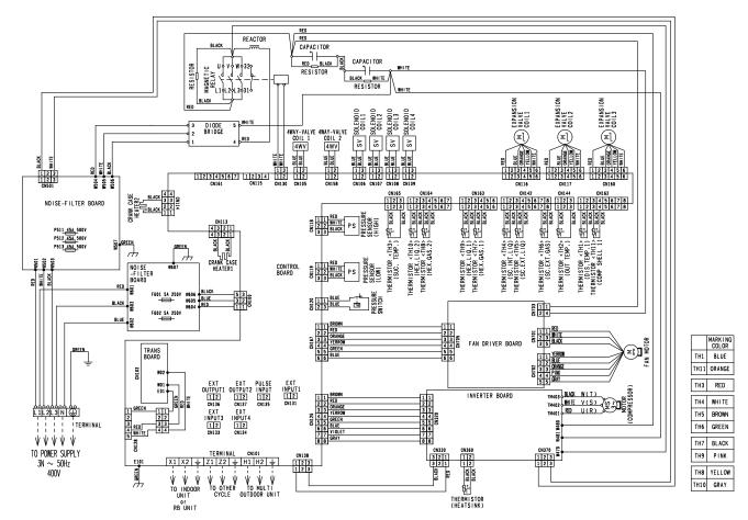
NOTE: • X1 and X2: To be connected to indoor unit or RB unit
