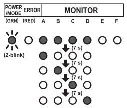
If the connection is incorrect (Example: When connection of B and C of the 4 units are reversed)
