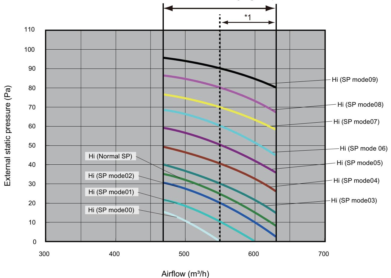
\*1: Available airflow rate range when Auto louver grille kit (option) is installed.
