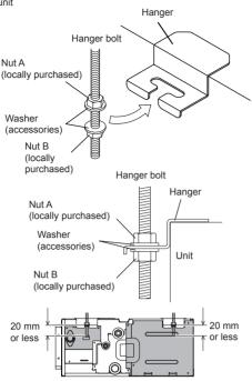
If the length of hanger bolt is over 20 mm, it will be not convenient for following works:
