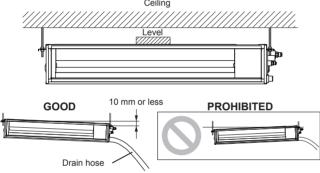
Give a slight tilt to the side to which the drain hose is connected. The tilt should be in the range of 0 mm to 10 mm.
