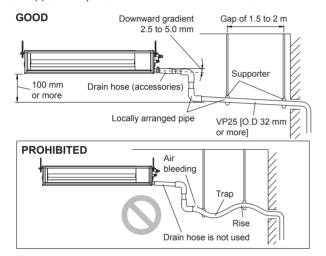
Observe the following procedures to construct centralized drain pipe fittings.
