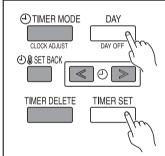
Press the DAY (DAY OFF) button and TIMER SET button simultaneously for 2 seconds or more to activate the child lock function and lock all of the buttons on the remote controller. Press the buttons again for 2 seconds or more to deactivate the child lock function.
