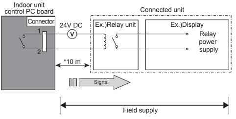
$^{\ast}$  Make the distance from the PC board to the connected unit within 10m. Relay spec. : Max.24VDC, 10mA to less than 500mA.
