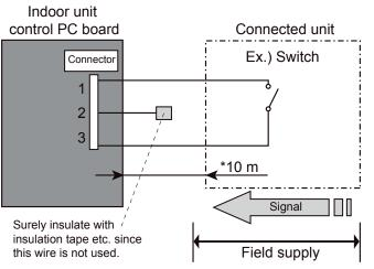
\* Make the distance from the PC board to the connected unit within 10 m. Contact capacity : 5VDC or more, 15mA or more. Please use non-polar relays and switches.
