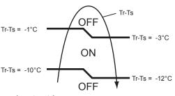
and Room Temperature(Tr) decrease below 19°C, signal output is on.
