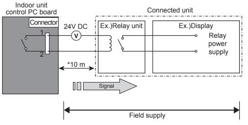
\* Make the distance from the PC board to the connected unit within 10m. Relay spec. : Max.24VDC, 10mA to less than 500mA.
