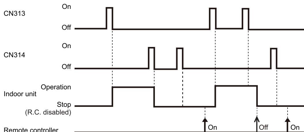
**NOTE:** When “Operation/Stop” mode 2 function is used with forming a remote controller group, connect the same equipment to each indoor unit within the group.
