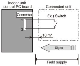
\*: Make the distance from the PC board to the connected unit within 10 m. Contact capacity: DC 24 V or more, 10 mA or more. Use the non-polar relays and switches.
