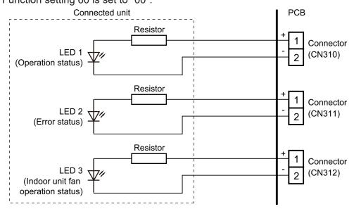
• When connecting with a device equipped with a power supply: Example: Function setting 60 is set to "00".
