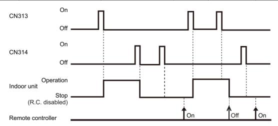
**NOTE:** When "Operation/Stop" mode 2 function is used with forming a remote controller group, connect the same equipment to each indoor unit within the group.
