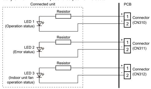
When connecting with a device equipped with a power supply:
