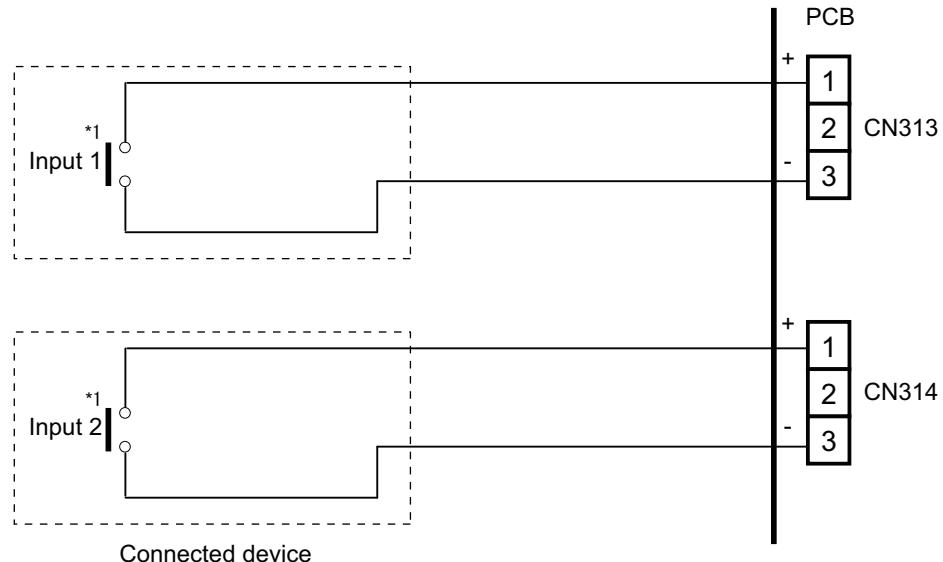
\*1: The switches can be used on the following condition: DC 12 V to 24 V, 1 mA to 15 mA.
