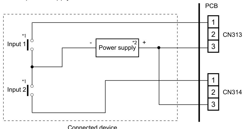
\*1: The switches can be used on the following condition: DC 12 V to 24 V, 1 mA to 15 mA.
