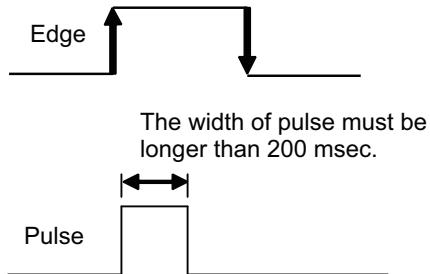
**NOTE:** The input signal supports the following switch type:
