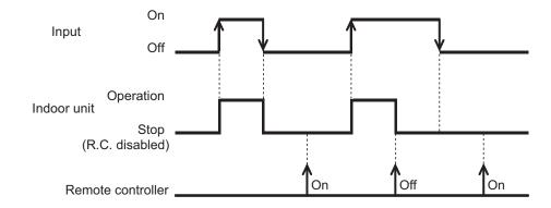
**NOTE:** When "Operation/Stop" mode 2 function is used with forming a remote controller group, connect the same equipment to each indoor unit within the group.
