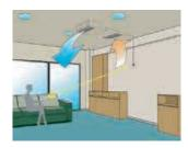
Duct type indoor unit can be controlled with Wireless remote controller if the IR receiver unit is used.
