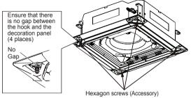
When there is a gap between the ceiling and the decoration panel even when the screw is tightened, readjust the height of the main indoor unit.
