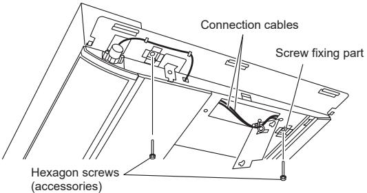
(17) Tighten the 4 hexagon screws you installed in steps (6) and (16), until the seal material between the Cassette grille and the indoor unit is compressed to a thickness of 5 to 7 mm (3/16 to 1/4 in).
