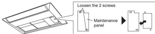
(15) Look through the maintenance opening to see if any cables interfere with the mount.
