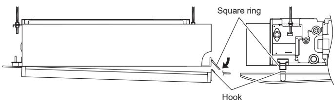
(14) Loosen the screws (do not remove) and remove the maintenance panel.
