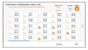
(2) There is a [Select (Delete)] button on the Confirmation of Registration Indoor units screen. When [Select (Delete)] button is tapped, [Delete] button appears and the screen moves to the Delete mode. The registered indoor unit can be deleted by checking the R.C.G..
