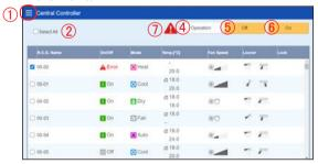
(1) Check the checkbox of R.C.G. to be changed for the setting.
