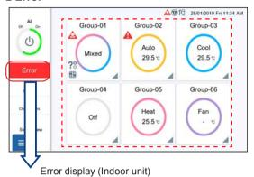
When the [Error] button is tapped, the error information (Error message or Refrigerant leakage) is displayed on the screen. Contact the service department as necessary.
