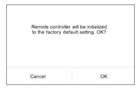
(4) When initializing this controller, tap the [OK] button. Wait for a while without turning off the power. After the initial setting screen appears, set according to the wizard. →Refer to 1-5.
