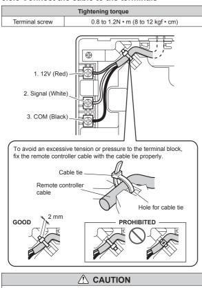
Be careful to avoid breaking the cable by over-tightening the cable tie. When connecting the remote controller cables, do not over-tighten the screws.
