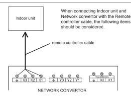
There are 2 methods to connect the remote controller cable to the indoor unit. One is the connection using contained connecting cable, and the other is the connection the remote controller cable is connected to the exclusive terminal block of the indoor unit.
