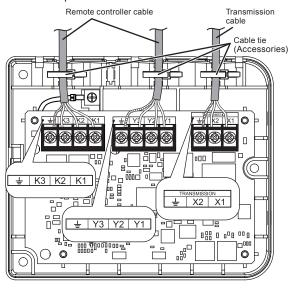
Fix the connector cable even outside the main unit as necessary. Fix the cable with cable tie using 3 fixing holes.
