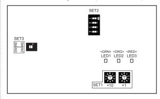
(1) [Rotary switch-SET1] set the refrigerant circuit address
