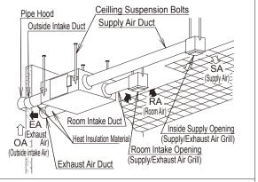
The two outside ducts(the Outside Intake Duct and the Exhaust Duct)must be insulated to prevent condensation. (Material; Glass wool, Thickness; 25)
