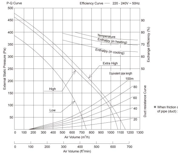
\* When friction coefficient of pipe (duct) :  $\lambda$ =0.02
