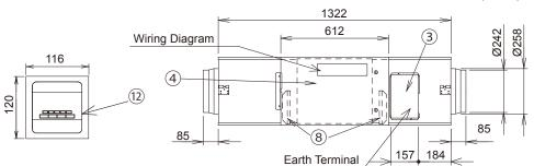
An inspection opening is necessary to clean the heat exchange element and filter once or twice a year.
